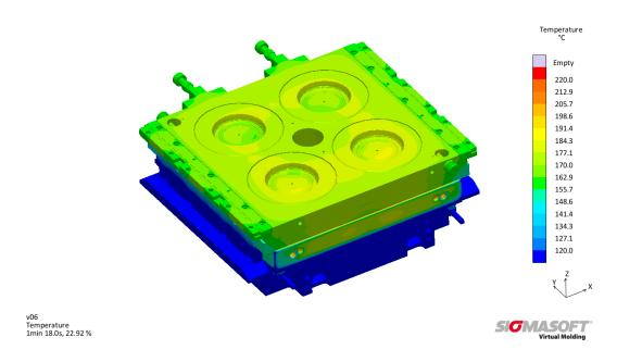
Figure 1 – To analyze the thermal mold layout, all components of the mold are taken into account and virtual parts are produced over several cycles to realistically reproduce the conditions of production
