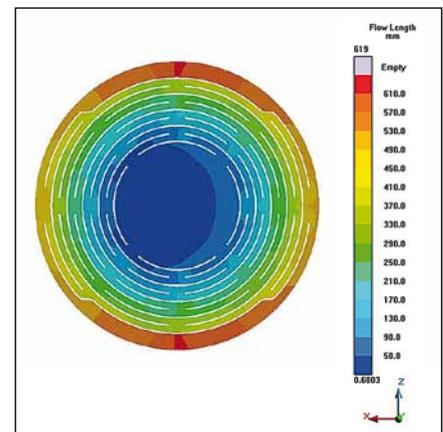
Figure 2: An interlaced geometry and a maximum flow length of 619 mm make the carry mesh challenging for production.
