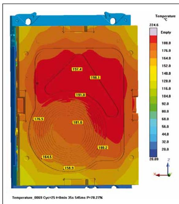
The reason for this varied outcomes is the temperature distribution inside the mold. While the classical approach assumes a homogenous temperature, the real mold shows quite high temperature variations. Taking a closer look on the moveable half after the thermal steady state is reached reveals that just inside the cavity the difference is already bigger than 30 °C (Figure 4).
