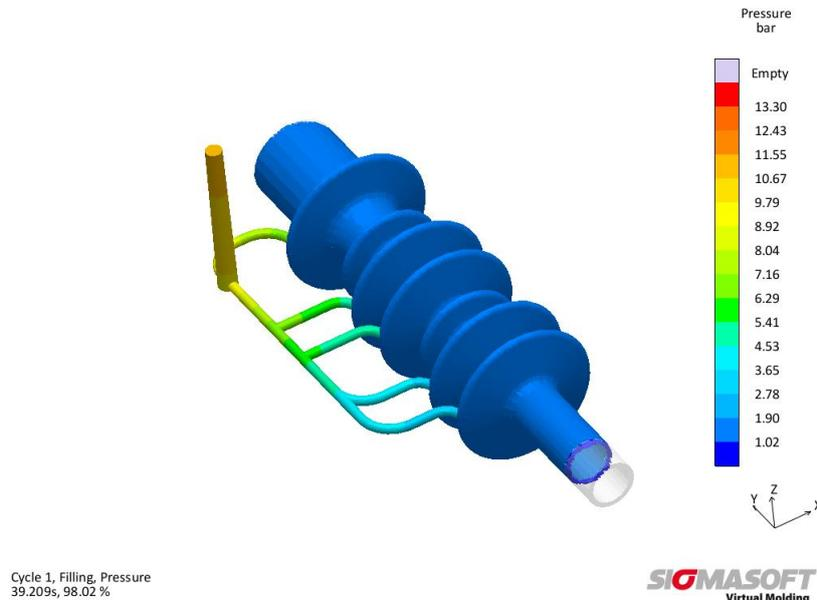
*Figure 2 – Pressure distribution in the virtually optimized version; the slightly increased pressure demand leads to a more balanced filling behavior*
