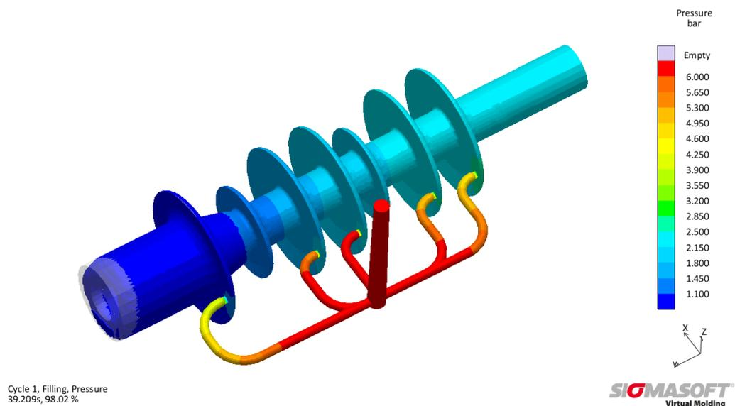
Figure 1 – Distribution of pressure while filling in the original design, the runner system causes a distinct unbalanced filling
