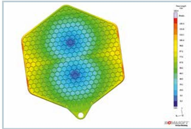
**Fig. 1.** The maximum flow-path length from the two injection points is 135 mm (orange/red on the color scale). The pot holder has a fine honeycomb structure with an averaged wall thickness of 1 mm (© Sigmasoft Engineering)
