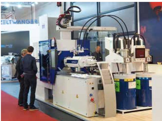
**Fig. 2.** The production cell developed by Wittmann Battenfeld combines a servohydraulic SmartPower 90/350 injection-molding machine and a pump and mixing unit from ACH solution on a compact footprint (© Hanser/F. Gründel)
