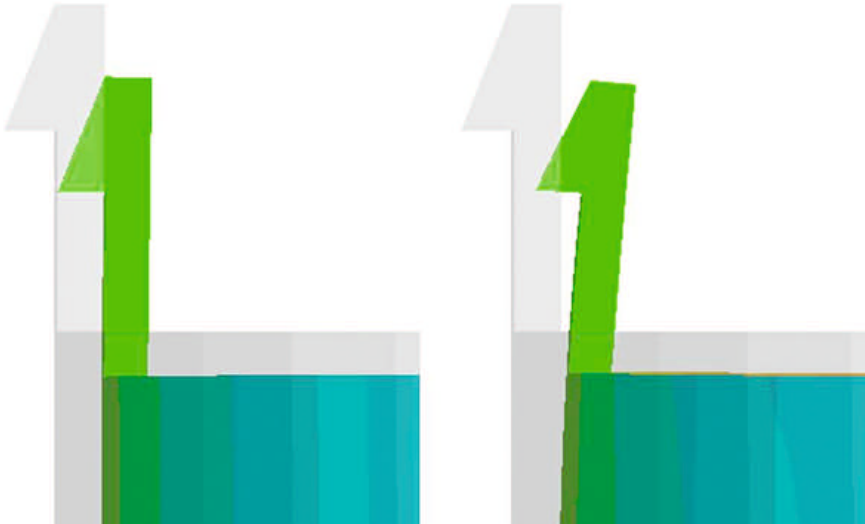
Fig. 3. If the heating of the mold is taken into account (right), the warpage of the part is much greater compared to a standard simulation (left) and agrees better with the real situation (figure: Sigma)
