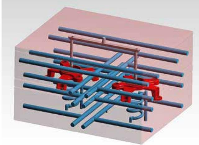
The detailed analysis of the filling-phase interactions having been completed, the thermal response of the mold during the holding and cooling phases was investigated. This entailed conducting a multi-cycle analysis of 20 consecutive virtual production cycles.
