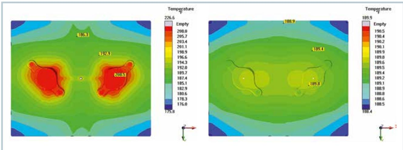
**Fig. 3.** Mold wall temperature: Cooling using a bubbler leads to hot spots (left) (see Figure 4) which can be eliminated by conformal cooling (right) (figures: Sigma Engineering)
