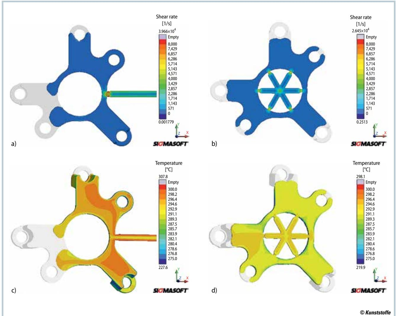
**Fig. 2.** Shear rate and melt temperature in a side-gate (a and c) are significantly greater than in a star-shaped gate (b and d) (figures: Sigma Engineering)
