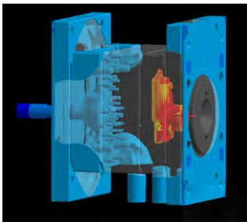
Sigma Plastic Services (Schaumburg, IL) highlighted this product at the recent NPE, where it says it was well received. The 3D-approach of Sigmasoft allows all the components in a mold, including all the thermal and physical properties of each one of them, to be reproduced. Therefore, the heat transfer process can be calculated between each one of the components.
