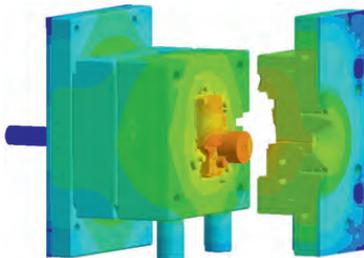
"In conventional injection molding software, a fixed mold temperature is defined, and the whole simulation is carried out under the assumption that this value remains constant over time," explained Marco Thornagel, executive director of Sigma Engineering.
